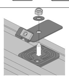
5. Attach all air deflector mounting plates to the stud plates with an M8 flat washer & nyloc nut.
