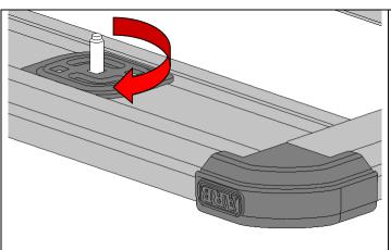
3. Flip the plate over and insert each of the four assembled stud plates into the front channel of the BASE RACK. Rotate 90 degrees and ensure the bolt on the two centre plate's lines up with the holes in the air deflector. The other 2 plates should be positioned near the ends of the channel.
