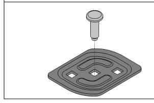
2. Insert one M8 x 25 Stud into each of the Stud Plates as shown.
