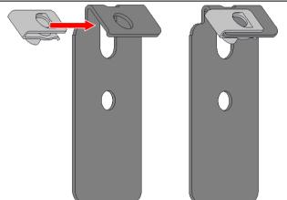
4. Snap one u-nut onto each of the air deflector mounting plates. Take care to ensure the u-nut is oriented correctly. See image.
