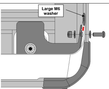
9. Place the large M6 washer (4581082) between the blade and the air deflector and secure using the remaining M6 Button head screws, M6 washers (4584329) and an M6 nyloc nut, as shown.
